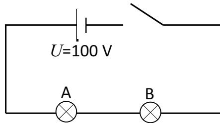
Consider the above circuit. The filament lamp A consumes an electrical power  $P_A = 100 \text{ W}$  when it alone is connected to a voltage of  $U = 100 \text{ V}$ . Filament lamp B consumes a power  $P_B = 20 \text{ W}$  when it alone is connected to a voltage of  $U = 100 \text{ V}$ .
