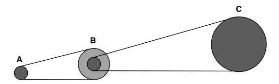
Pulley A rotates at a rate of 8 complete turns every second. If the belts do not slip, then how many complete turns every second will pulley C make?
